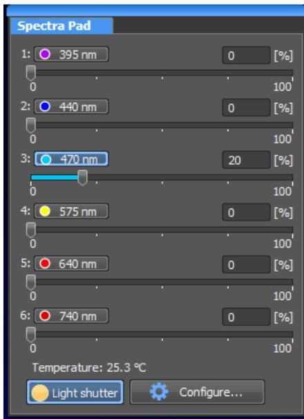
The **Spectra Pad** controls the LED light source for image acquisition. Selecting the wavelength such as 470 highlights the tract and selecting the **Light shutter** button at the bottom of the tab activates the light source. The light power percentage can be adjusted using the slider or by typing into the box.
