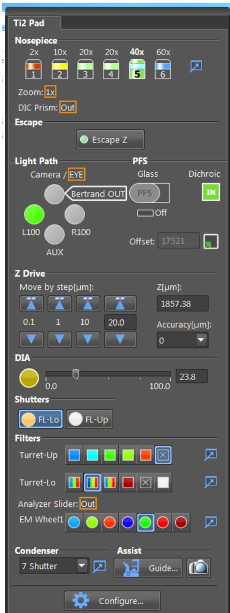
Under **Nosepiece** are the available **objectives**. Placing the arrow over each objective will provide information.
