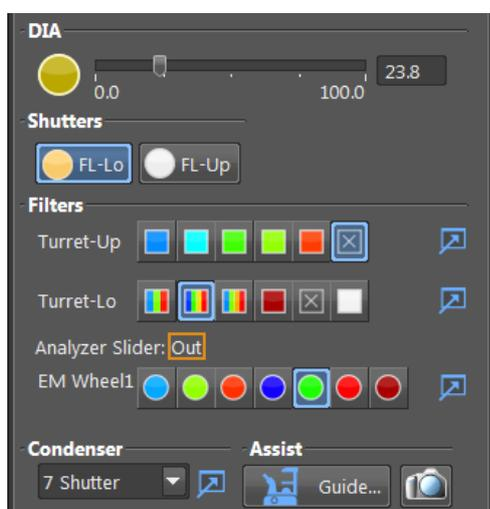
Check that the **correct shutters** are open and that **unused filter** are not in the way and.
