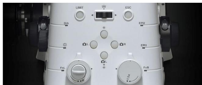
*Buttons on microscope body*
