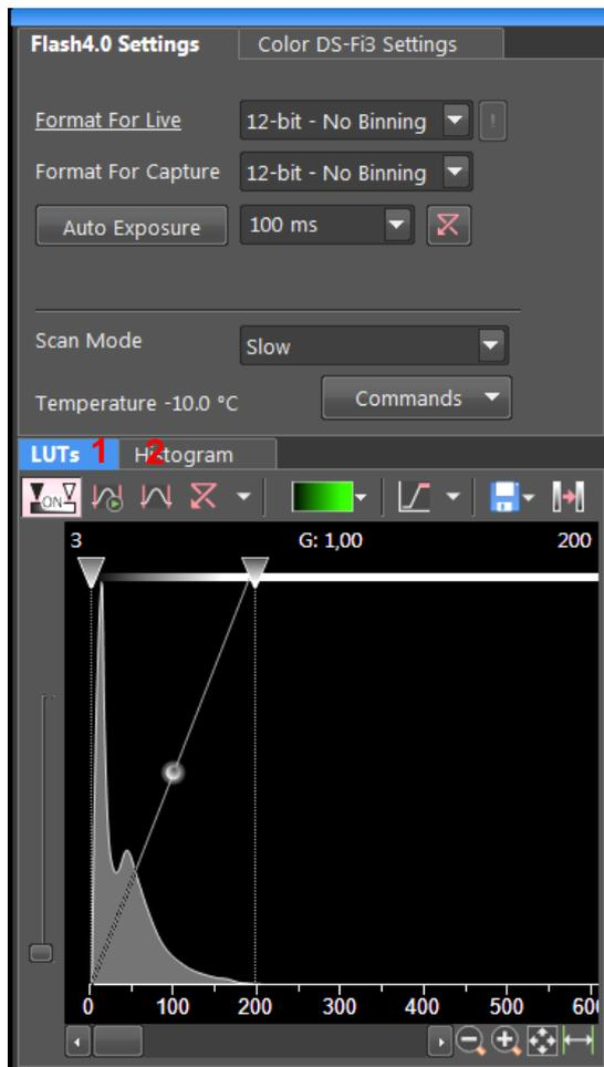
As previously mentioned, exposure time and binning can be modified in the camera setting windows.
