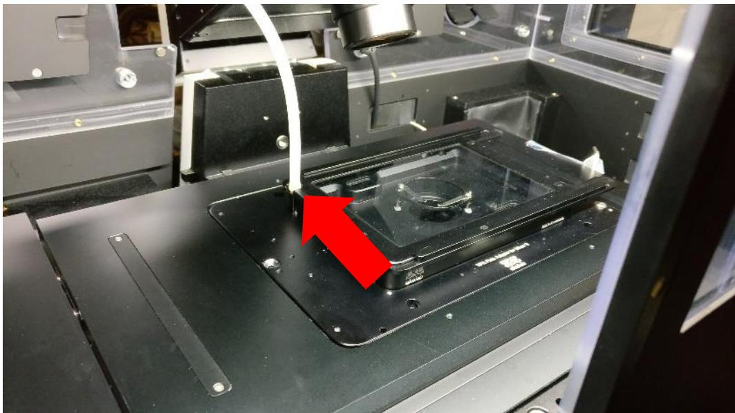
Note: Make sure to connect the air tube (arrow) into the imaging chamber so the CO<sub>2</sub> reaches the cells.
