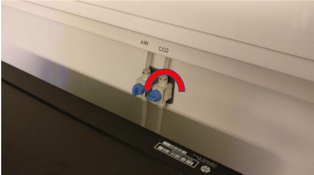
Just before imaging, switch the CO<sub>2</sub> on (at the wall beside PC) by turning the valve counter-clockwise to vertical position. Then adjust the CO<sub>2</sub> setting on the Okolab controller.
