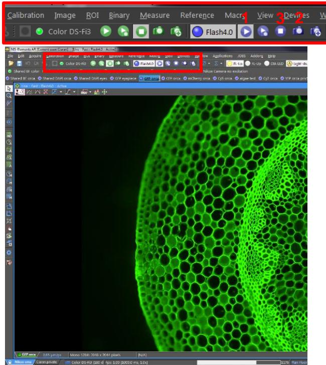
The visualisation window is where the camera can be activated to obtain a live image of the sample.
