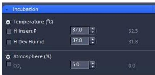
Switch on/off the incubator and CO<sub>2</sub> through the software. Typically, 37°C and 5% CO<sub>2</sub> are used for normal cell imaging.
