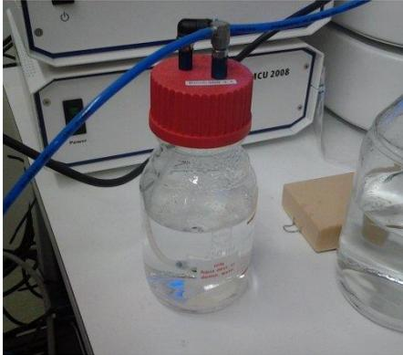
Check that there is distilled water in the humidifier bottle.
