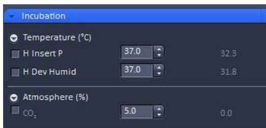
Switch on/off the incubator and CO<sub>2</sub> through the software. Typically, 37°C and 5% CO<sub>2</sub> are used for normal cell imaging.
