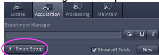
The **Smart Setup** function allows you to insert your fluorophores and the software will provide light path suggestions.
