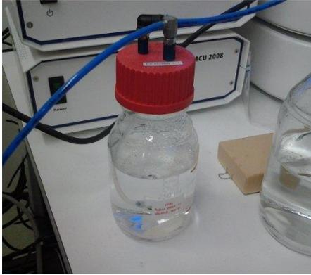
Check that there is distilled water in the humidifier bottle.
