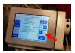
**NOTE:** the first user must open the RL shutter on the touchpad to allow fluorescence through the eyepieces!
