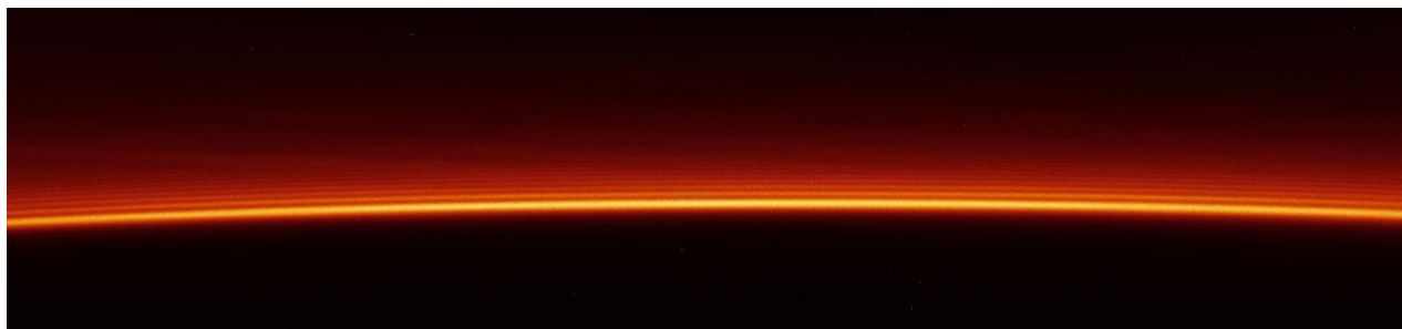
Figure 2.1 - The Airy beam illumination profile that defines the Aurora Light Sheet system.
