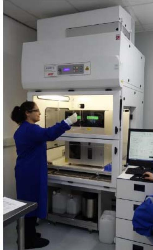
The CAS Cabinet Class II Biosafety Cabinet is custom build for the Sony SH800. There is an easy access door on the front panel for convenient chip loading, as well as a side door on the left side for re-filling the DI tank which is used for flushing the sample line between the samples.
